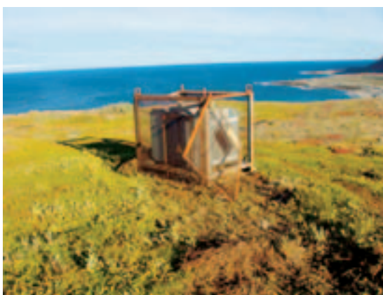
Figure 4. RTGs positioned along the Russian coast (Photo: Office of the County Governor of Finnmark).
