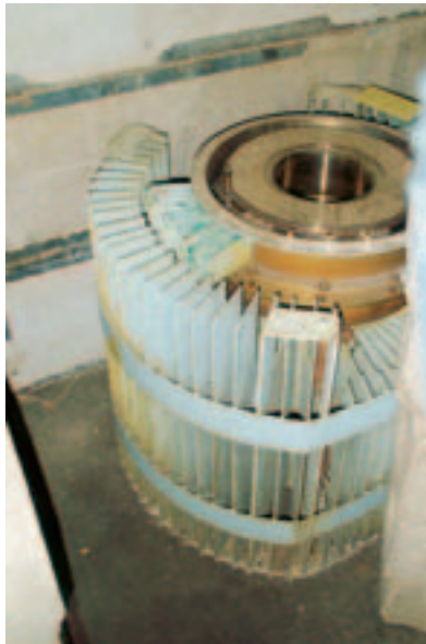
Figure 1b: Photograph of a typical RTG (with ^{90}\text{Sr} heat source removed) (Photo: NRPA).
