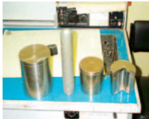
Figure 2. Example casings for the ^{90}\text{Sr} heat source. On the right-hand side the casing is cut away to reveal where the ^{90}\text{Sr} would be held (Photo: NRPA).
