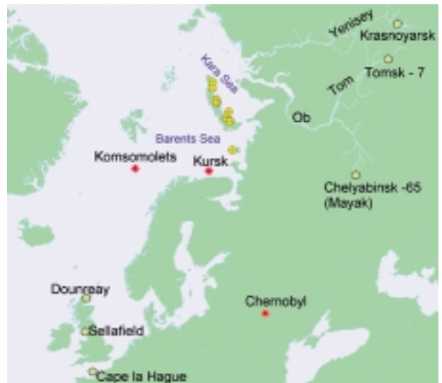
Fig.2.4 Sources of radionuclides in to the northern marine environment: Chernobyl in the Ukraine, the reprocessing plants at Sellafield, La Hague and Dounreay, the dumping sites of nuclear waste in the Kara Sea, the sunken submarines Komsomolets and Kursk and Russian nuclear installations (Mayak, Tomsk-7 and Krasjonoyarsk-26) releasing radionuclides to the Russian rivers Ob and Yenisey.
