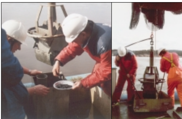
Photo 3.2, B. K. Føyn: Collection of sediment samples in Iddefjord, onboard G.M. Dannevig (IMR) in 2001.
