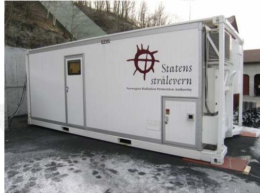
*Figure 4. NRPA's mobile laboratory applied in the monitoring of reindeer herders*
