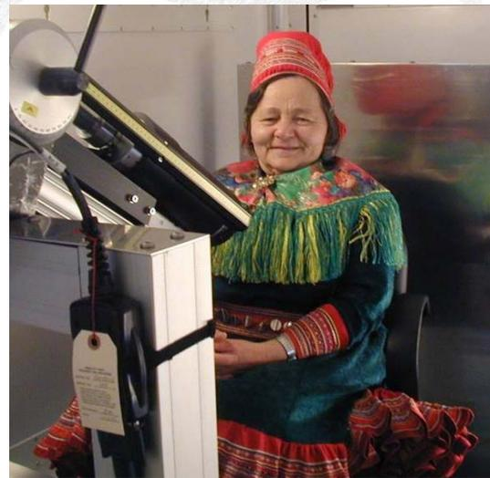
*Figure 5. Measurement of body content of caesium-137 in a Kautokeino lady in 2005*
