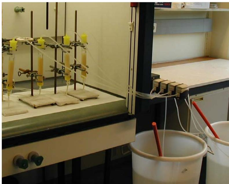
**Figure A.1.** 50 litres of sea water is passed through an ion-exchange column.
