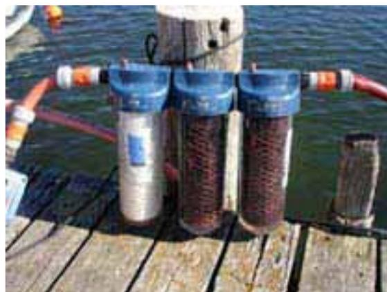
**Figure 3.2.** Filter system used for analysis of  $^{137}\text{Cs}$  in sea water.
