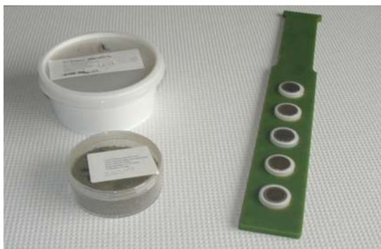
**Figure A.2.** Dried sample material in different containers ready for gamma measurements. To the right,  $^{99}\text{Tc}$  preparations ready for counting.
