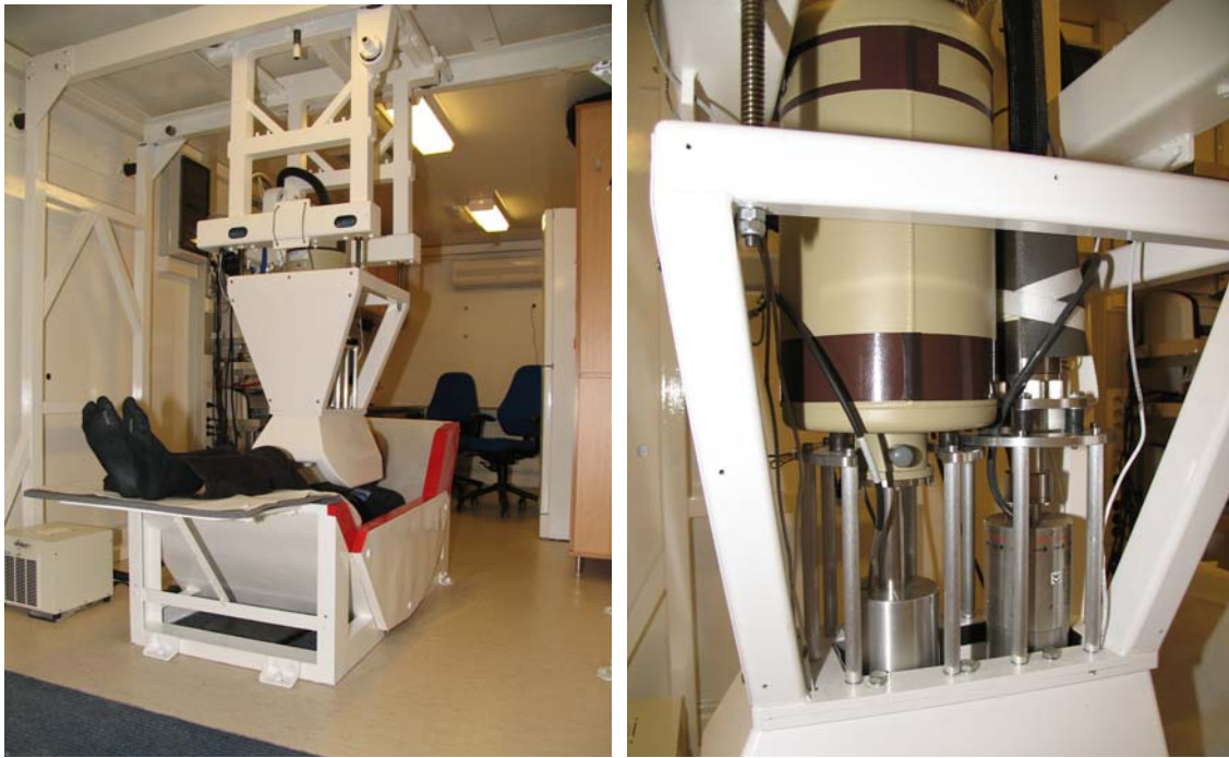
Figure 2 Left: Inner view from the truck. Right: The two HPGe-detectors
