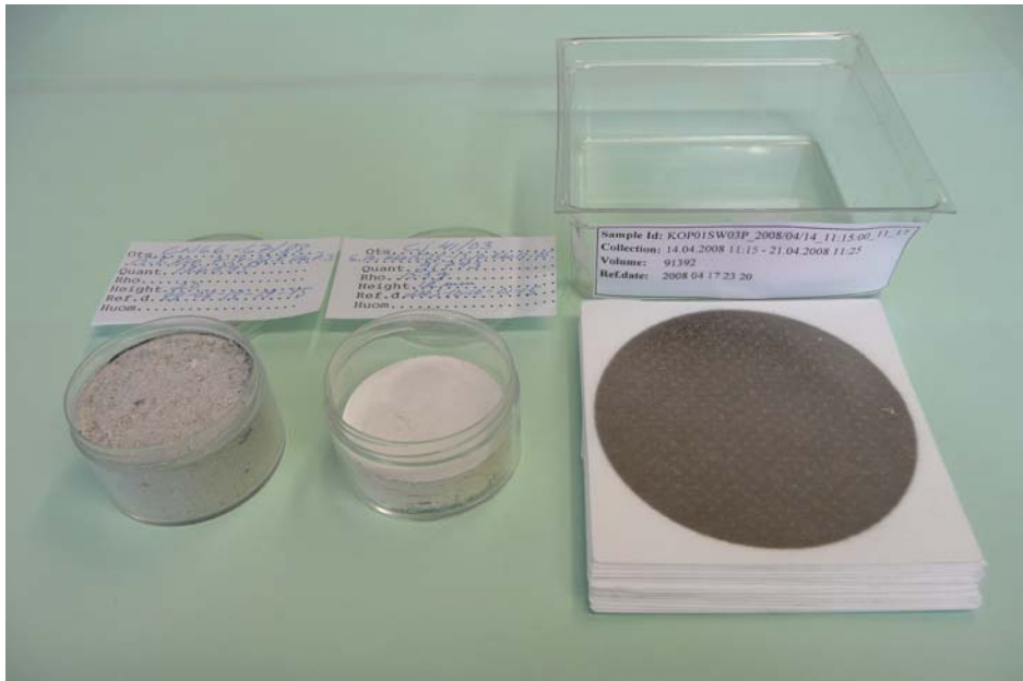
Figure 1. Air samples in the past and today. The traditional way of processing air filters for counting is to press the sample to the smallest possible volume. However, the original sample is destroyed making it difficult to perform any other studies. The counting efficiency is reduced very little in a geometry with larger diameters (77 mm filter, 80 mm detector, BEGe5030). The filters are not destroyed and subsamples suit further studies, such as ordinary alpha spectrometry or measurement with PANDA.
