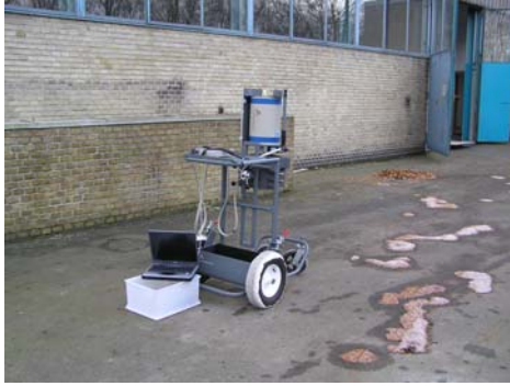
Figure 2. Clearance measurements on the area around the reactor building using a germanium-detector for measurements on asphalt and grass surfaces.
