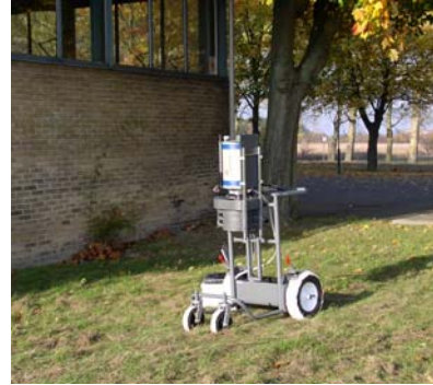
Figure 2. Clearance measurements on the area around the reactor building using a germanium-detector for measurements on asphalt and grass surfaces.
