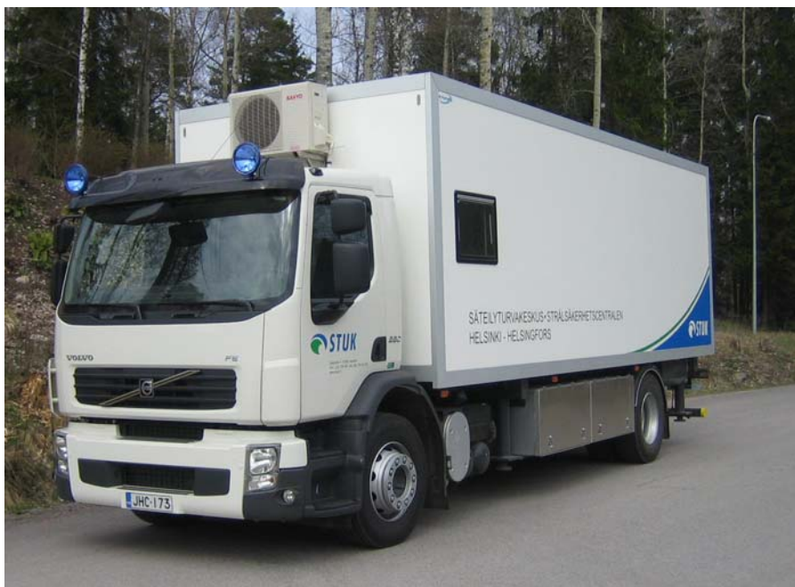
Figure 1 A new mobile whole-body counter.
