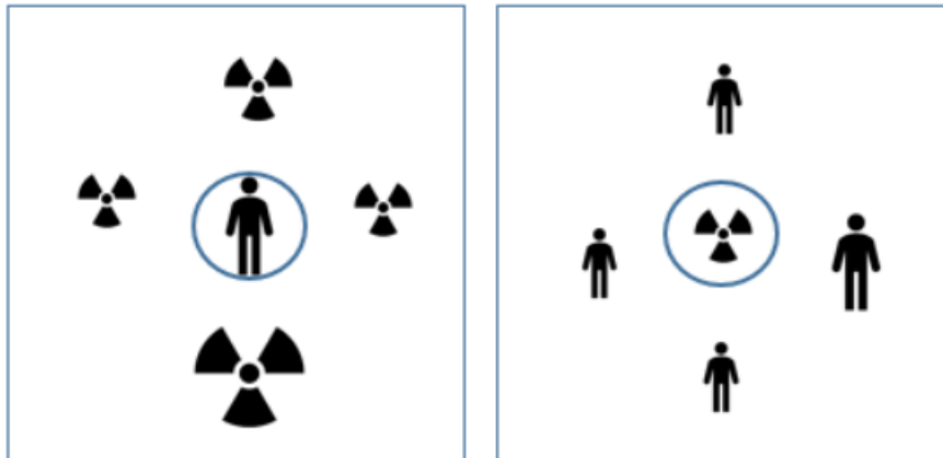
Figure 2.1. Illustration of the difference between dose limits that apply to a specific person (left) and dose constraints that apply to a radiation source (right).
