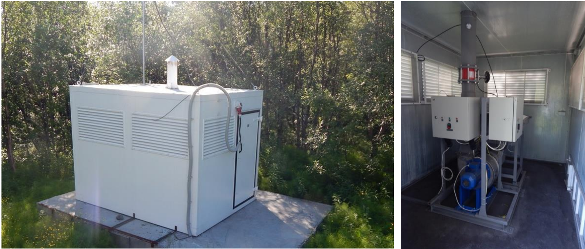
Figure 2: The Murmansk sampling station for radioactive contamination of the ground air. The shelter and the air sampling instrument inside. Photo: Murmansk Hydromet
