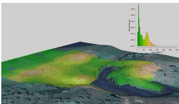
Three dimensional mapping of  $^{137}\text{Cs}$  along a floodplain in the PSRER.
