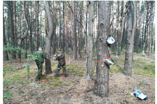
Joint DSA – PSRER field work in developing field methods for assaying trees for contaminants.
