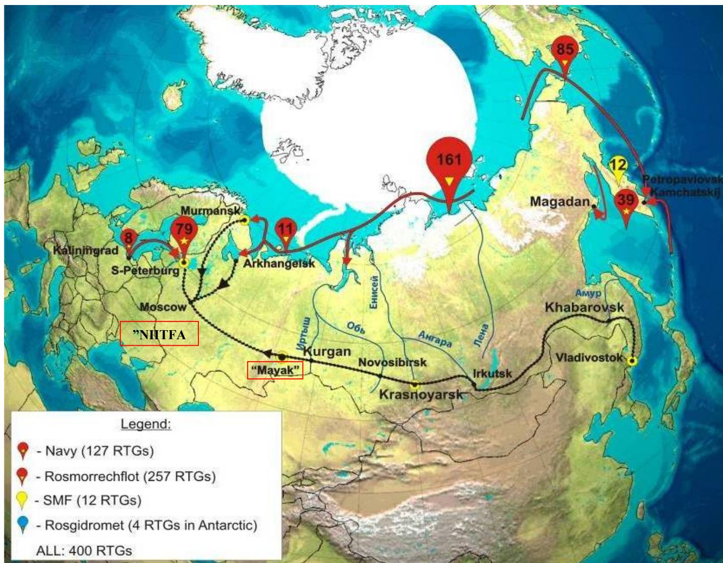
**Figure 4.** A schematic map of the remaining RTGs in the territory of the Russian Federation showing the transport routes from the site of removal (red, yellow and blue markers) to the dismantling (NIITFA) and disposal (Mayak PA) facilities (Kurchatov Institute, June 2009).
