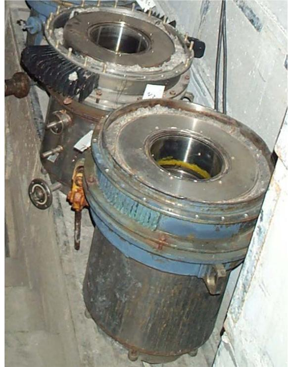
Opened RTGs (with the Sr-90 heat sources extracted) stripped of cooling fins at NIITF (Photo: NRPA).
