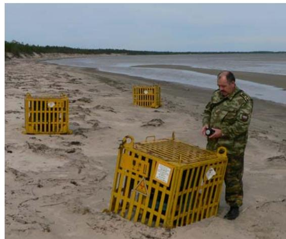
*Measurement of radiation doses during inspection of a RTG in Northwest Russia (Photo: County Governor of Finnmark).*
