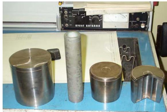
Different types of casings for pellets (Sr-90 heat source) extracted from RTGs as well as a cut-away showing where the Sr-90 pellets are held (Photo: NRPA).
