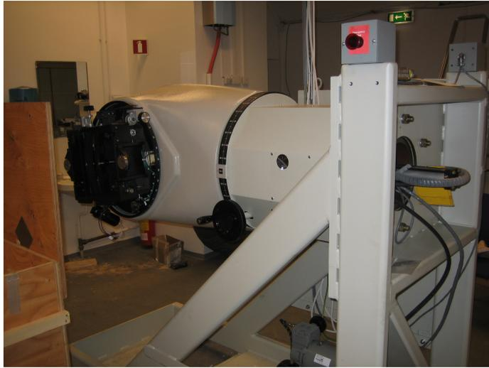
Figure 8: Co-60 Gammatron at the NRPA. Photo taken by Hans Bjerke.
