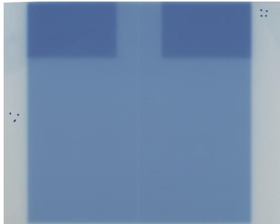
Figure 19: Typical example of an exposed GafChromic® EBT film. The film has been exposed to two 200 MU 10x20 cm<sup>2</sup> fields as well as two 200 MU 5x8 cm<sup>2</sup> fields.
