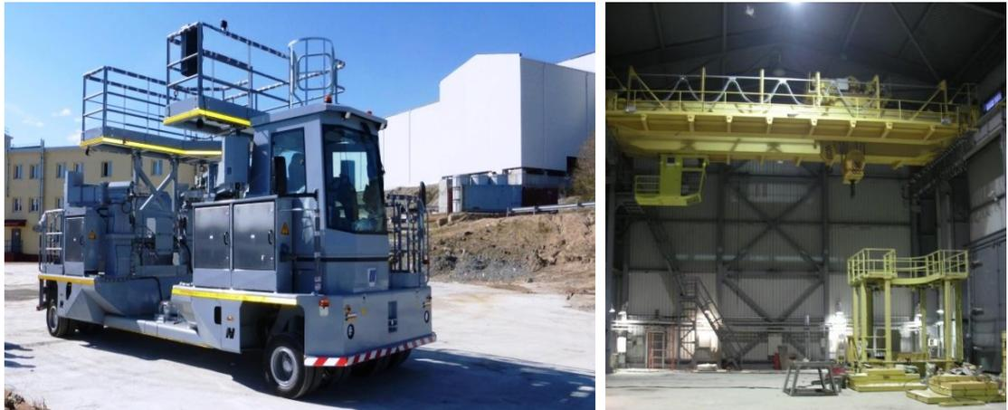
Fig. 2. Left: Transporter container carrier for TPC-108/1 (TC-18) transportation from Building 153 to Building 151, right: rail transfer truck and bridge crane.
