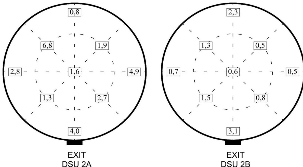
Fig. 6 Gamma dose rate inside DSU's 2A and 2B, μSv/h.
