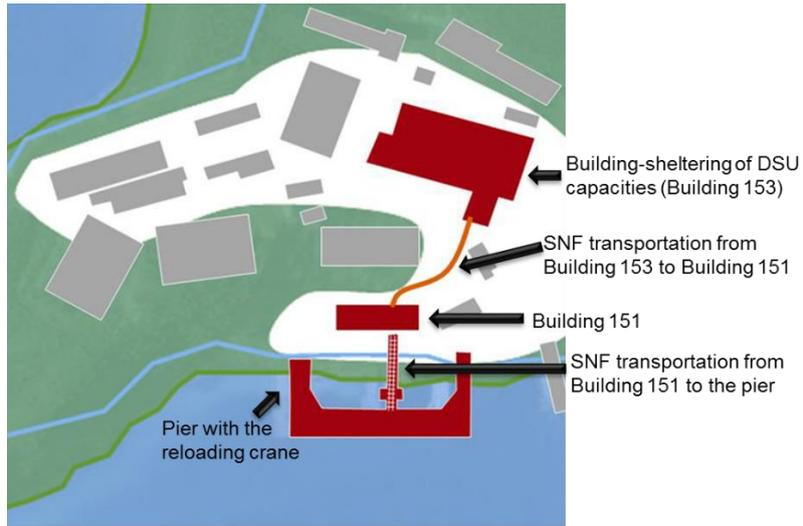
Fig.8 Technological plan of the SNF removal from the Andreeva Bay NWC SevRAO site [1]
