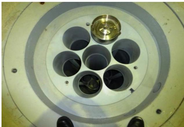
Fig. 4C The unit of the case loading (changing the cases) consists of cells for 7 cases
