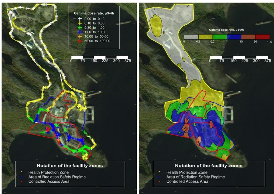
Fig. 39 Dot map of gamma survey results over 2015 (left). Contour map of gamma survey of the Andreeva Bay SevRAO site over 2015 (right).
