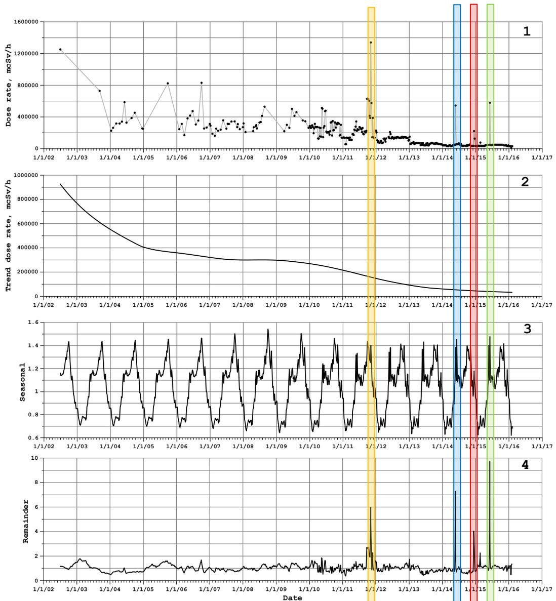
Fig. 14 Decomposition of the time series of the AEDR integral over the technical site at Andreeva Bay over the period 2002-2016. 1- initial time series, 2- trend, 3- season, 4- remainder components of the initial time series.
