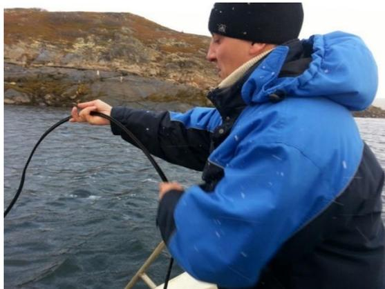
Fig. 41 Measurement by the near bottom gamma spectrometry method aboard a boat.
