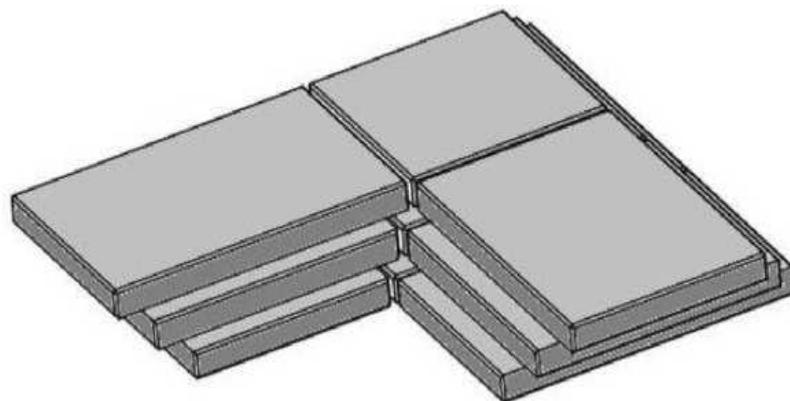
Fig.5 Segments of the horizontal biological shield [2]
