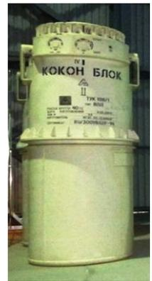
Fig 9. Reloading unit (RU) installed in Building 153, Reloading protective container for SFA, Transport package container
