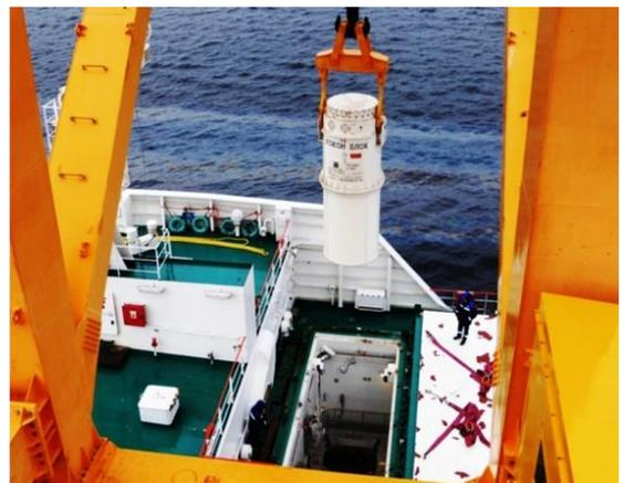
Fig. 10. Overhead crane with lifting capacity of 50 tons, installed on the pier, loading of the TUK into the cargo compartment of the "Rossita" ship
