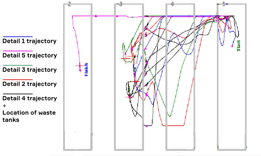
Fig. 32 Path of movement of the crane. Sign "+" shows the position of barrels containing waste.
