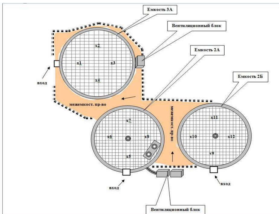
Fig.7 Location of points of measurement of gamma dose rate at the site of DSU location
