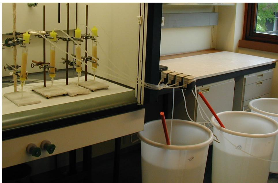
*Figure 2. Technetium is separated from sea water by ion exchange chromatography.*
