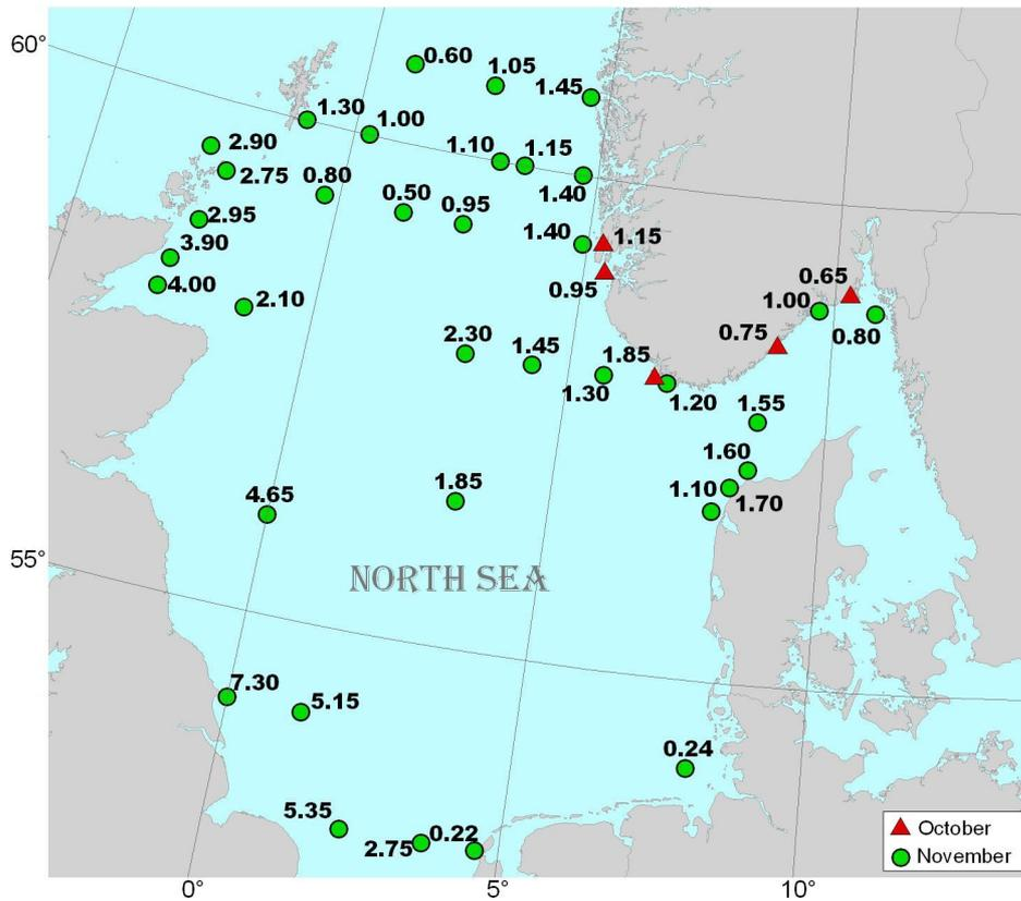
**Figure 5.** Concentrations of <sup>99</sup>Tc (Bq m<sup>-3</sup>) in surface sea water samples collected in the North Sea, 2001.
