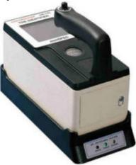
Gr-135 - "The Identifier". Handheld instrument for the identification of any finds or sources.
