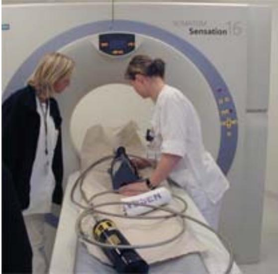
**Figure 3.2.** Computerised tomography of detector T3
