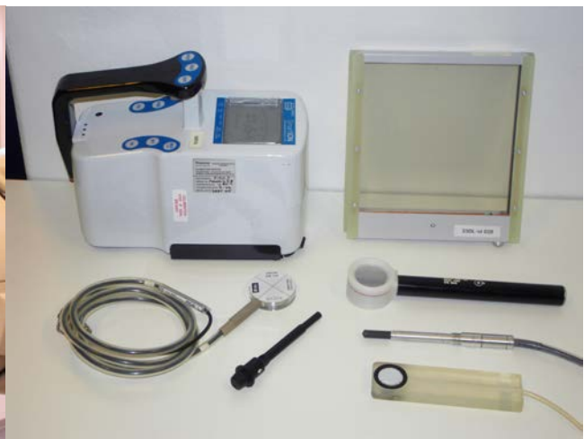
Calibration of reference chamber for radiotherapy dosimetry. Collection of units under test.
