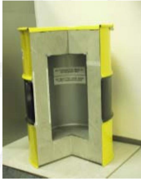
*Section of a steel drum encased in concrete.*
