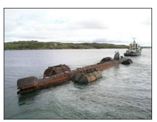
K-159 under tow on the way out from Gremikha in 2003 with floatation pontoons. Photo: The Russian Northern Fleet.
