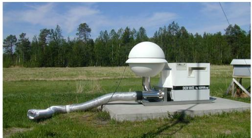
Air filter station at the Norwegian Radiation Protection Authority's Preparedness Unit at Svanhovd in Finnmark County.
