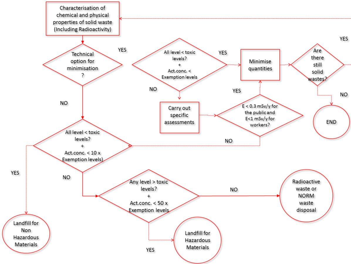
Figure 2. Decision framework for the disposal of NORM waste in Spain.
