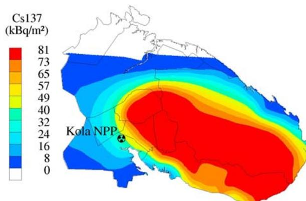
Figure 2. Worst case scenario for deposition of radiocaesium in the Murmansk region, calculated by DMI.
