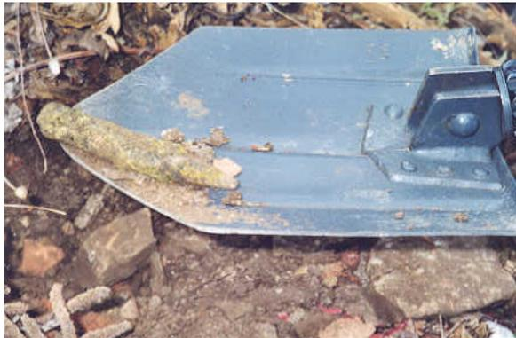
*Projectile made of depleted uranium*
