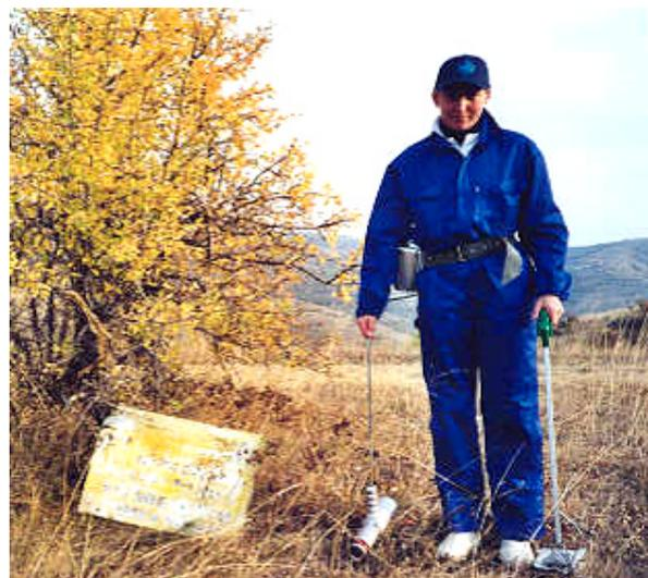
*NRPA representative with instruments for measuring gamma and beta radiation*
