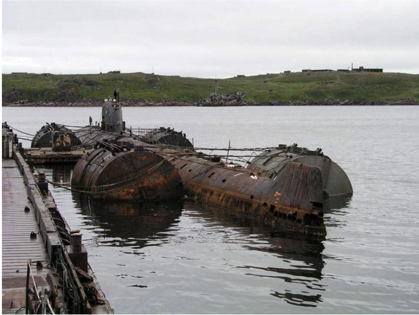
*Figure 1.2. The nuclear submarine K-159 with the four floatation pontoons strapped to it prior to being towed. Photo: The Russian Northern Fleet.*
