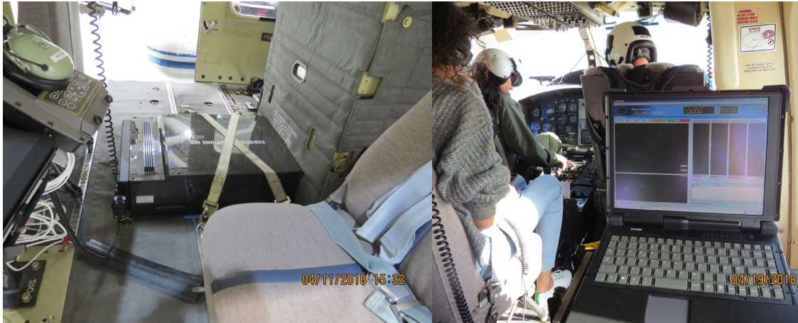
FIGURE 10. INTERNALLY MOUNTED RSI DETECTOR AND SUPPORT SYSTEM. ON THE LEFT ARE THE TWO RSX-1 CRYSTALS AND RSN-4 NEUTRON DETECTOR, AND ON THE RIGHT IS THE CONTROLLING LAPTOP. EQUIPMENT WAS STRAPPED TO TIE DOWNS IN THE AIRCRAFT.
