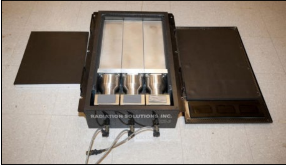
FIGURE 3. RSX-3 BOX WITH THREE 2" X 4" X 16" NAI(TL) CRYSTALS.
