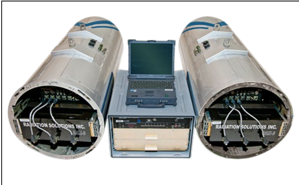
FIGURE 2. AMS RSI SYSTEM COMPONENTS.
