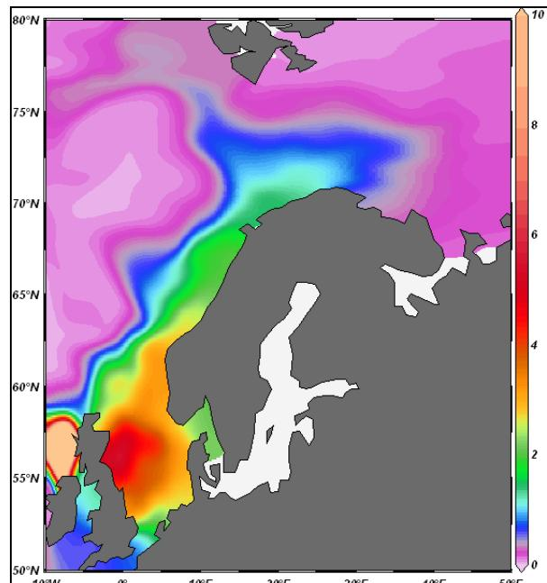
Modelled long range transport of  $^{99}\text{Tc}$  from Sellafield to the Norwegian Arctic by ocean currents produced through collaboration with AWI/OASys, Germany.
