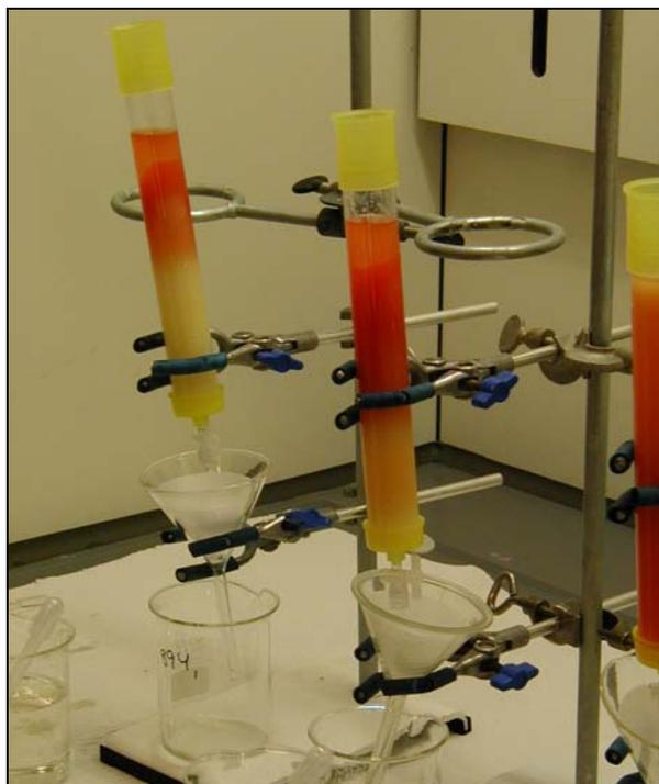
*Ion-exchange separation of <sup>99</sup>Tc from sea water samples collected in the Norwegian Arctic.*
