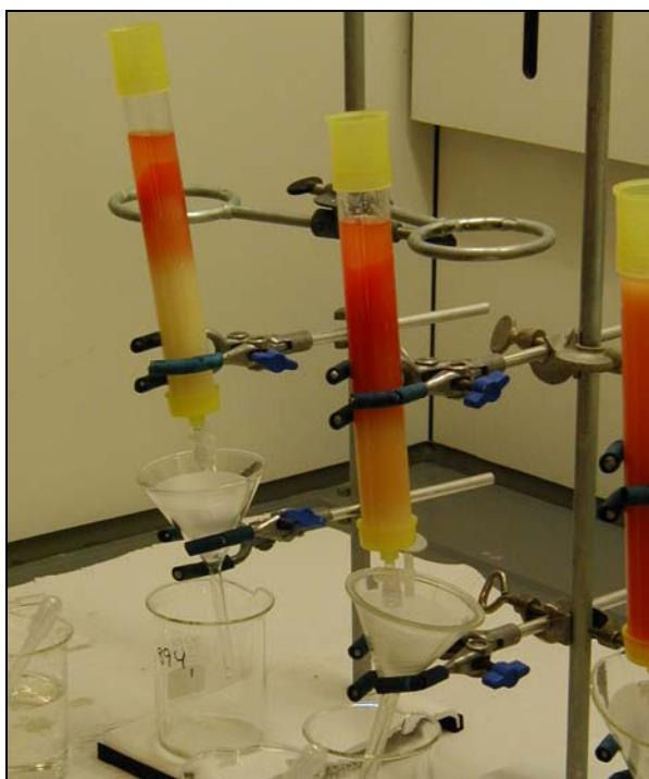
*Ion-exchange separation of  $^{99}\text{Tc}$  from sea water samples collected in the Norwegian Arctic.*
