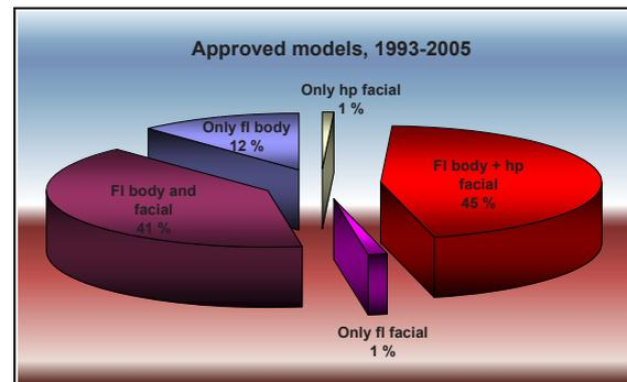
Figure 1. Distribution of the approved tanning models in Norway with respect to type and combination of fluorescent (fl) and high-pressure (hp) lamps.
