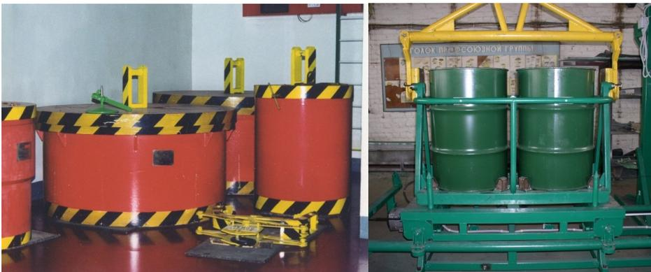
Fig. 4.2 Radioactive material in packages fixed for transport in a container
