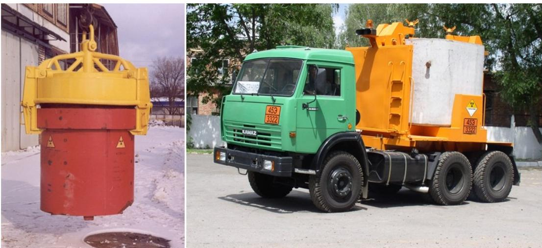
Fig. 4.4 Equipment for radioactive material transport
