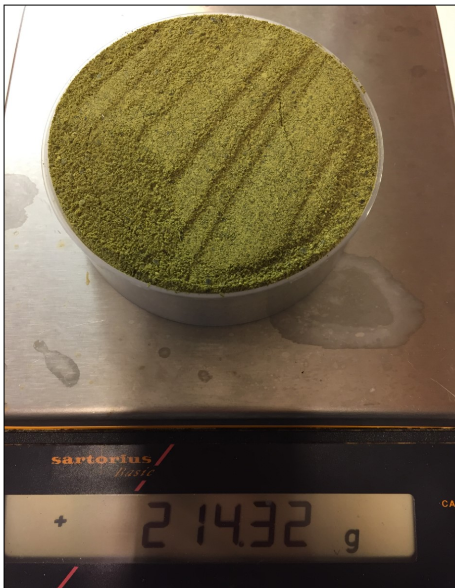
Figure 16. Dried and homogenised sample of Fucus vesiculosus ready for gamma-spectroscopy. Photo: Hilde Elise Helda, IMR.
