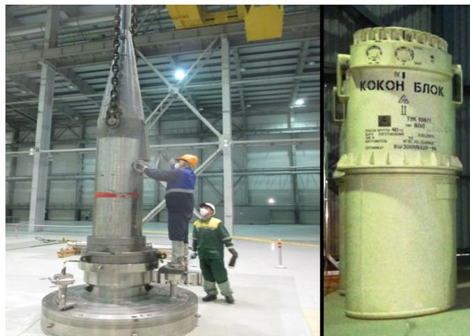
**Fig. 3 Reloading container for SFA (left). Transport package container (right) (source: SRC-FMBC).**
