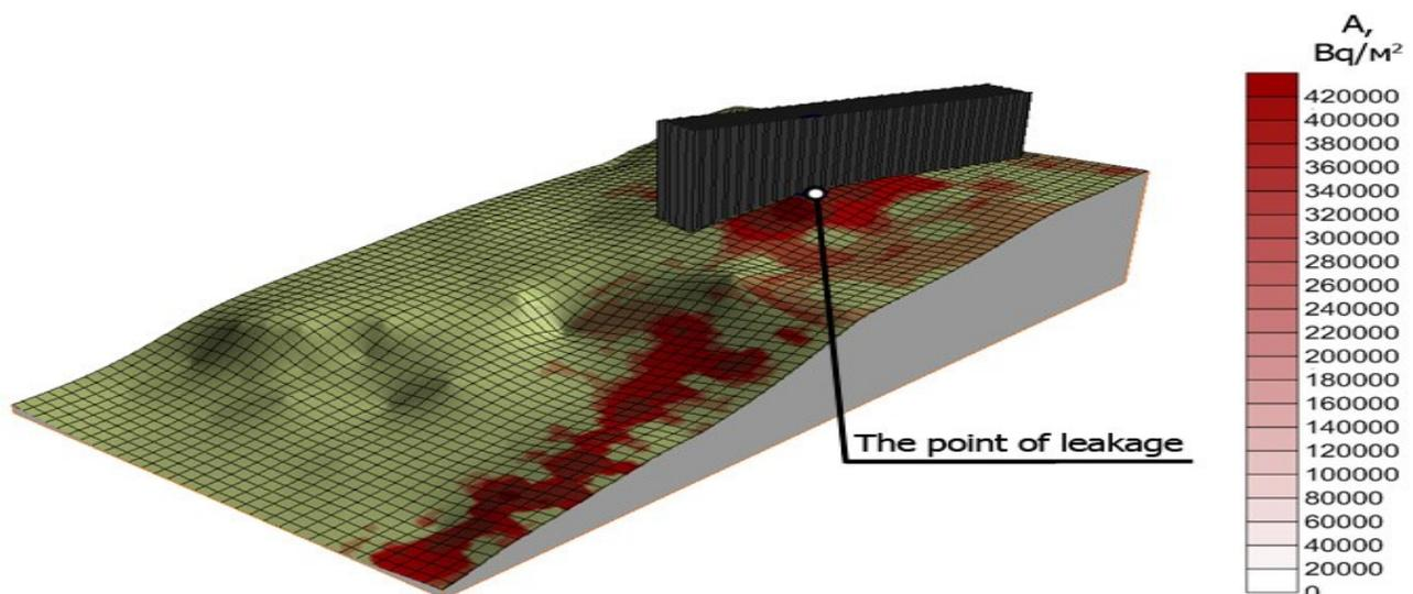
Fig. 1 Three-dimensional model of the distribution of surface activity in the area of the stream flowing out from under Building No. 5, Andreeva Bay STS (source: SRC-FMBC).
