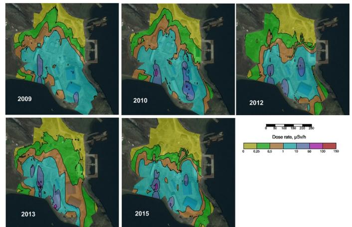
**Fig. 7 Dynamics of gamma dose rate at the industrial site over 2009-2015. (source: SRC-FMBC).**
