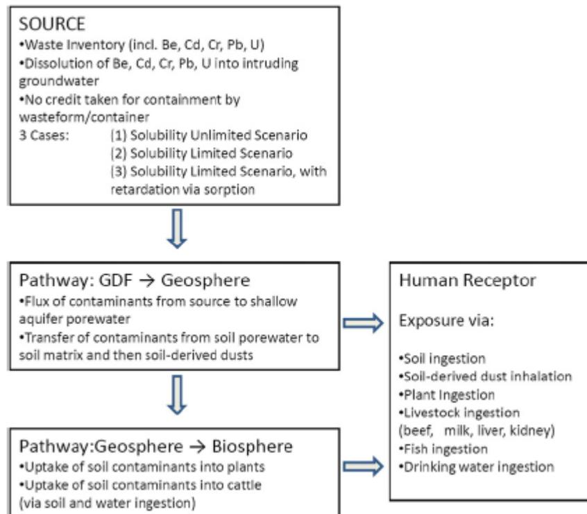
Figure 3-5. Schematic diagram of the approach taken by Wilson et al. (2009, 2011) to assess risks to human health posed by chemotoxic species in a generic UK Geological Disposal System.
