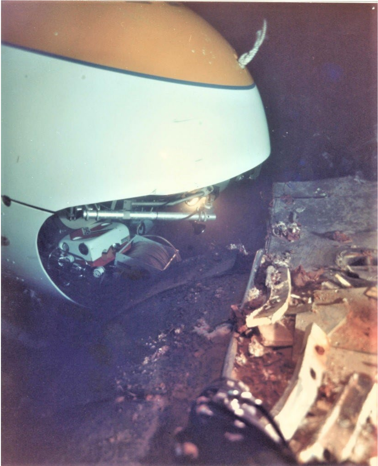
Figure 1.5. Photo showing one of the MIR submersibles investigating damage to the torpedo compartment of Komsomolets during the 1993 Russian investigation. The photo's perspective is taken looking away from the bow of the submarine and shows the starboard side of the torpedo compartment before this area was covered with tarpaulins. (Photo: DSA).
