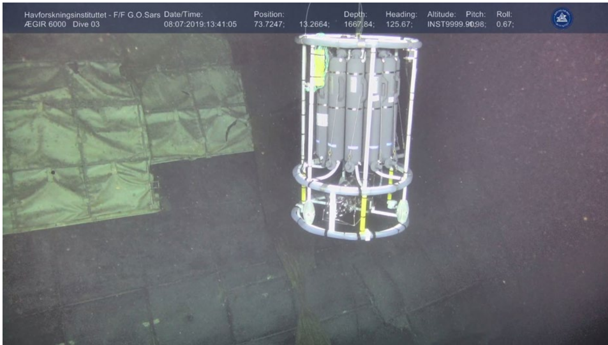
Figure 2.2. Large volume samples collected around 3 m directly over the ventilation pipe (upper photo) and next to the opening in torpedo compartment on the port side of the submarine (lower photo) (Photos: IMR).
