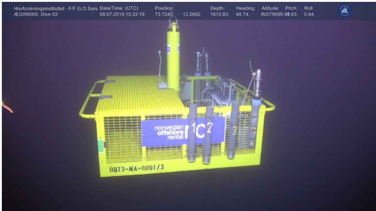
Figure 2.6. Auxiliary basket used in conjunction with the ROV to return sediment samples to the surface (Photo: IMR).
