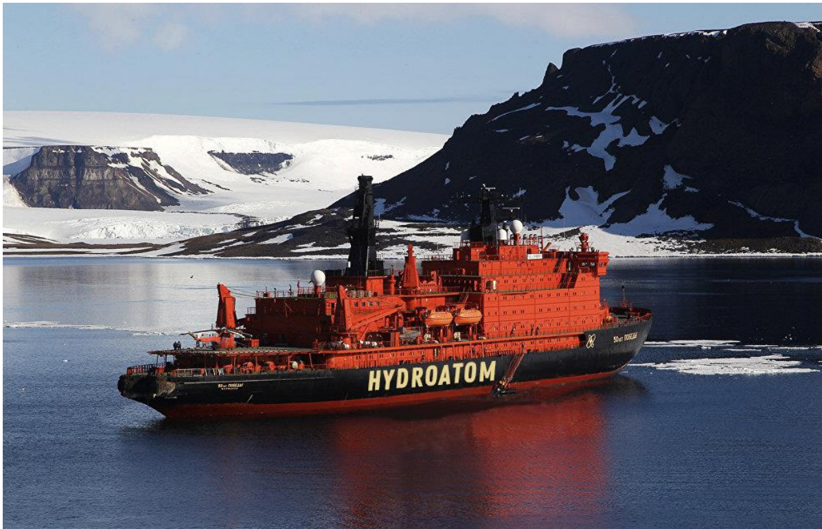
Figure 2: The icebreaker HYDRATOM. The vessel has two 171 MW t reactors using high enriched (90%) U/Zr cladding as fuel. The vessel had 128 cruise passengers and a crew of 140 persons on board from four nationalities: Canada, USA, UK and the fictitious nation of Atlantistan, used as the vessel's nationality in the Arctic REIHN exercise.
