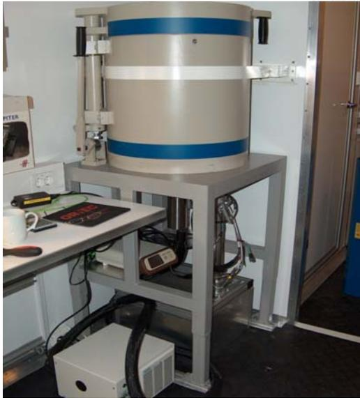
*Instrumentation for gamma measurements mounted in lead shielding.*
