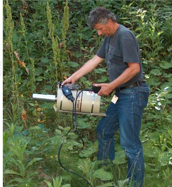
*Portable high resolution gamma detector for field usage.*
