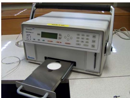
*Portable instrumentation for measuring alpha and beta radiation in contaminated sample materials.*
