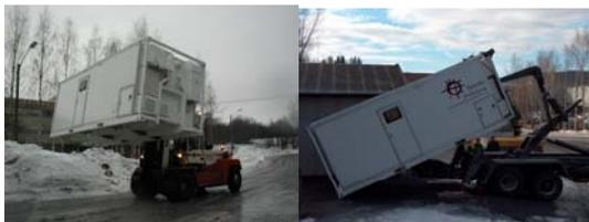
*The container can be raised by various means.*
