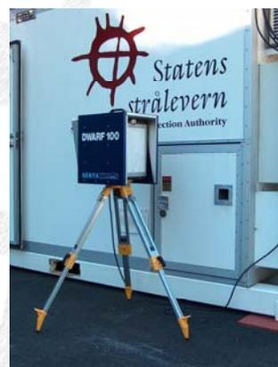
*Equipment for sampling of soil and sediment (to the left) and a portable air sampler for measurement of airborne radioactive contamination (to the right).*
