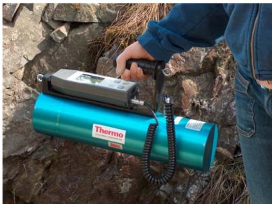
*Dose rate monitor with probe for differentiation between natural background radiation and anthropogenic radioactive contamination.*
