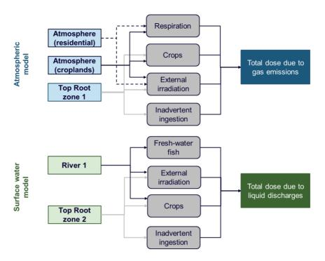
**Figure 3-12.** Relevant compartments for the estimation of the dose to public in the atmospheric and surface water model.
