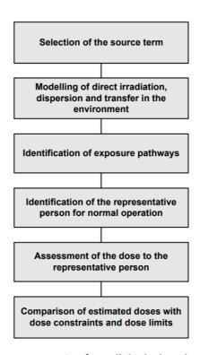
**Figure 3-1.** Scheme showing the components of a radiological environmental impact assessment for protection of the public in normal operation [9].
