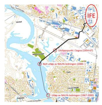
*Figure 5-6.* Location of the NALFA pipeline, discharge point of the liquid wastes from the IFE-Kjeller facilities.
