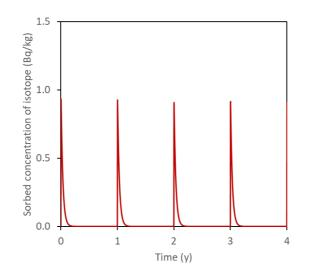
*Figure B. 3.* Evolution of the I-131 concentration sorbed in the soils during the first 4 years of the operational period under the continuous atmospheric emission scenario.
