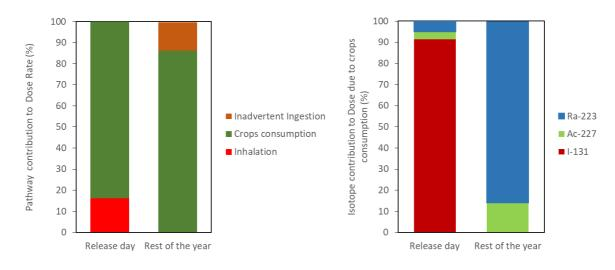
*Figure 6-5.* Pathway contribution to the dose rate the day of the total acute release and the rest of the year (left) and the contribution of the main isotopes to the exposure via crops consumption (right).
