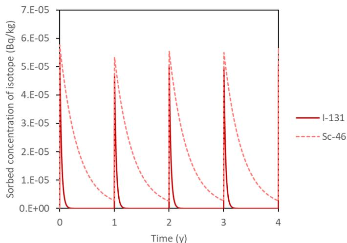
**Figure B. 3.** Evolution of the I-131 and Sc-46 concentration sorbed in the soils during the first 4 years of the operational period under the total acute atmospheric emission scenario.
