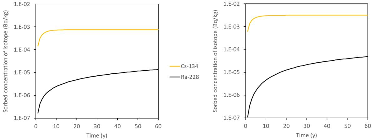
**Figure B. 4.** Evolution of the concentration sorbed in the soils (left) and sediments (right) during the operational period under the continuous atmospheric emission scenario.
