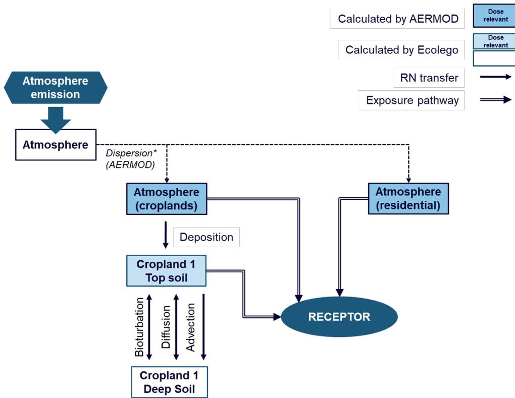
Figure 4-2. Conceptual model for the atmospheric emissions.
