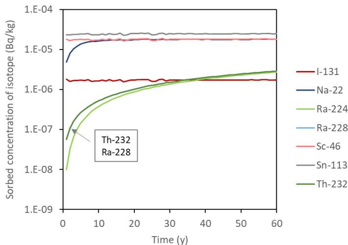
**Figure B. 2.** Evolution of the concentration sorbed in the soils during the operational period under the continuous atmospheric emission scenario.
