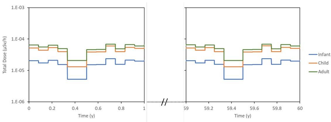
**Figure 6-1.** Evolution of total dose rate with time for each exposed age group under the continuous atmospheric emission scenario.
