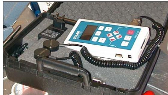
The spectroradiometer and the broadband radiometer with UVA and UVB sensors used during the inspection surveys.
