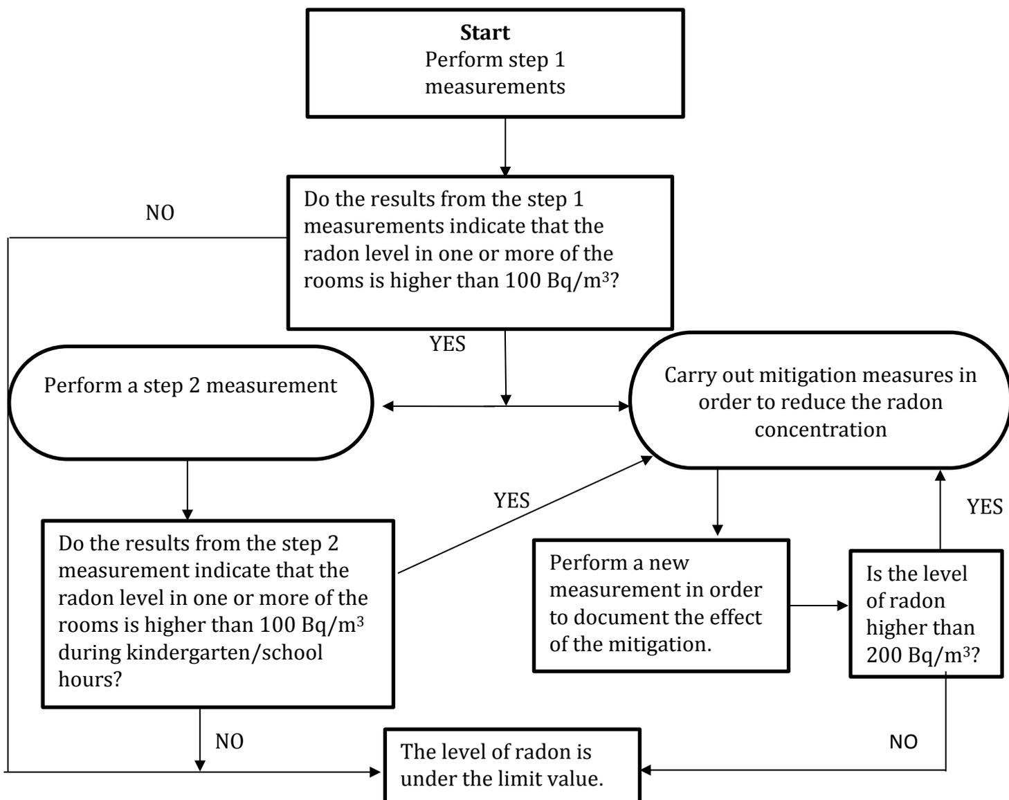
**Figure 1:** Flow chart illustrating the principals for measuring radon in schools and kindergartens
