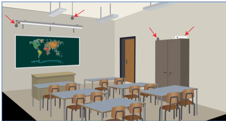
Measurement devices can be placed on the teachers' desk. Alternatively etched track detectors in step 1 measurements can be hung on a cord or placed on the top of a cupboard. On the top of a cupboard is also suitable for measurement devices in step 2 measurements.
