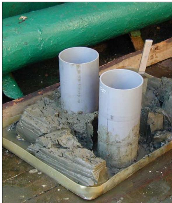
*Collection of sediment profiles from the box-corer.*
