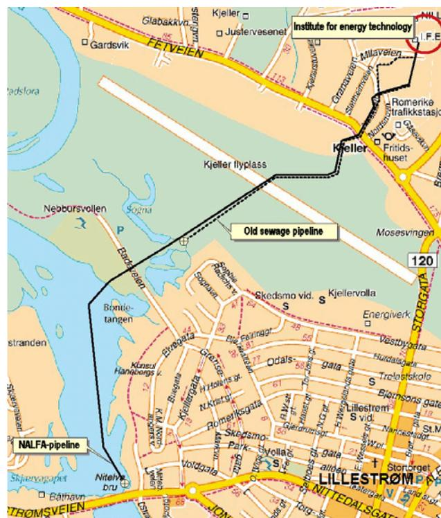
**Figure 2.1.** Map showing discharge pipelines from the IFE Kjeller facilities. The old pipeline was used until 1967. In 2000, the waste outlet was moved and part of the NALFA pipeline is no longer used and has been removed.
