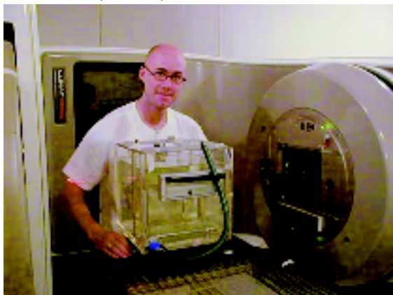
Figure 33 Ståle Ølberg placing the water phantom in the beam at UUS.
