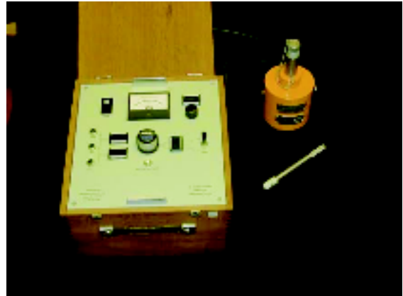
Figure 5 NPL Secondary Standard consists of chamber, electrometer and check source.
