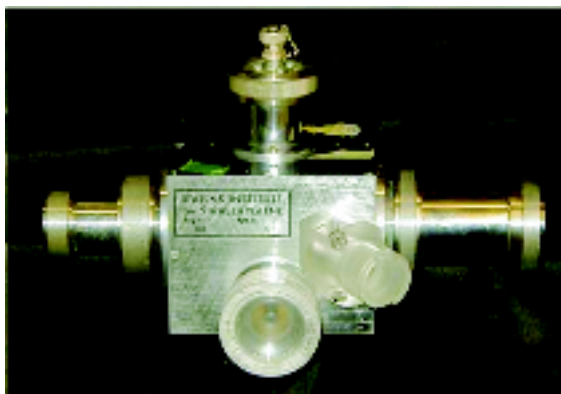
Figure 4 Free air chamber for low energy x-rays. Primary standard in Norway from 1960 to 1980.
