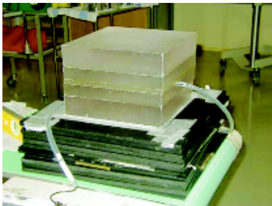
Figure 26 The polystyrene phantom in use at HUS.
