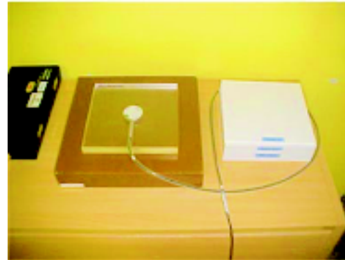
Figure 31 Polystyrene phantom for routine measurements in electron beams.
