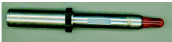
Figure 3 Vicoreen 100r chamber.
