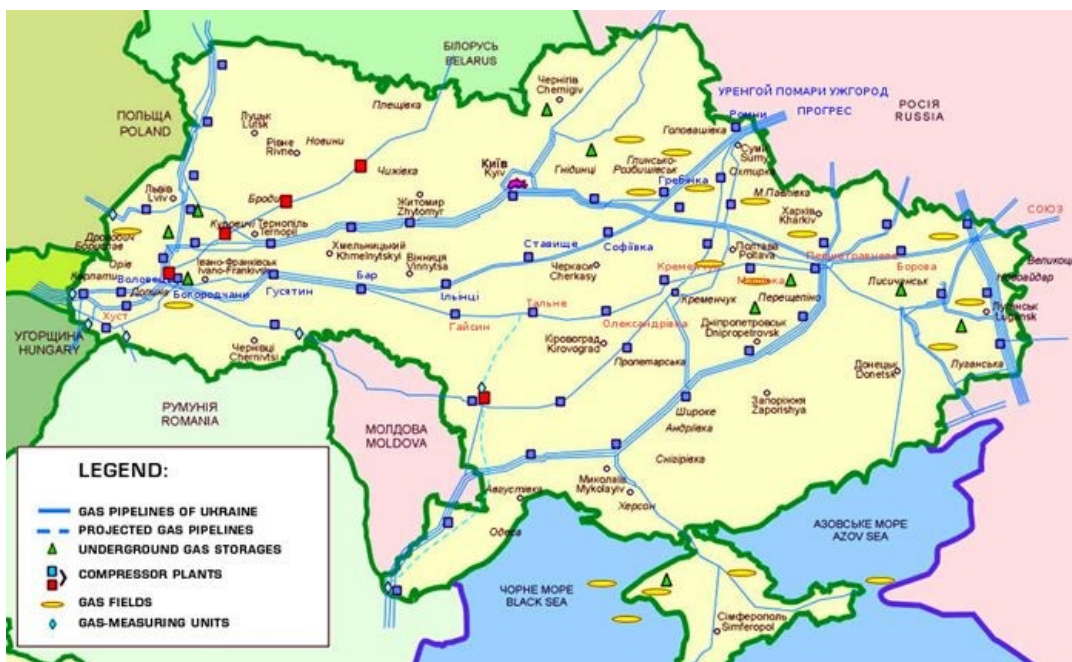
Figure 6.4 –Location of gas fields, gas metering and compressor stations, underground gas storages in Ukraine
