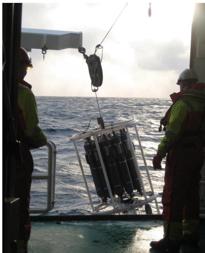
Figure 3.4. Sea water sampling with a CTD/Rosette multi-bottle sampler (Photo: Hilde Skjerdal, NRPA).
