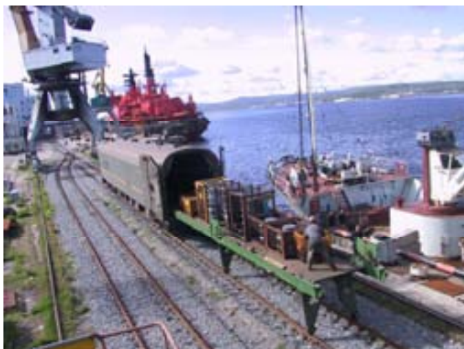
Fig. 9. Unloading of the ship with delivered RTG packages and their putting on the extension platform of a special railcar at FSUE Atomflot.
