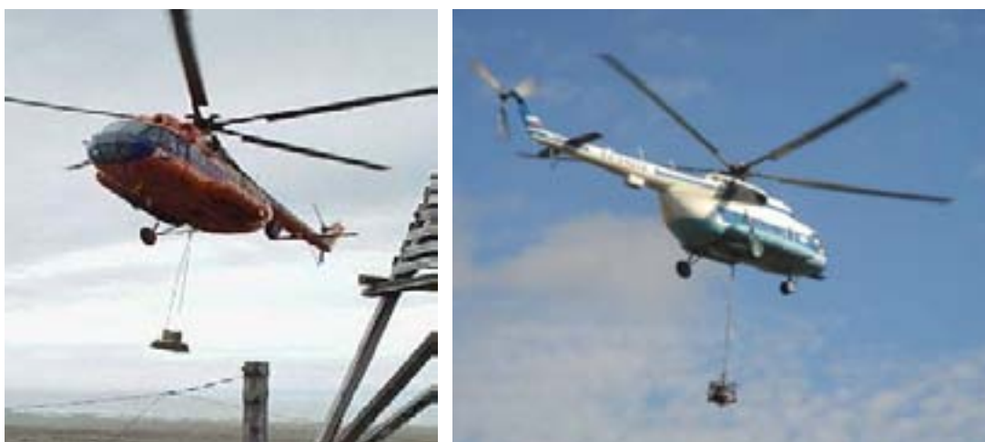
Fig. 8. The transportation of the dismantled RTGs from their installation locations to the coastline where it is possible to place them on a pontoon.
