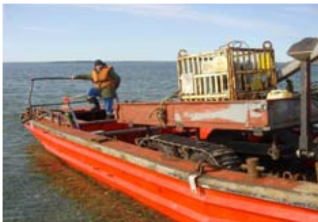
Fig.5. The decommissioned RTG package is placed on pontoon (for delivery to ship). The pontoon personnel should be minimal.
