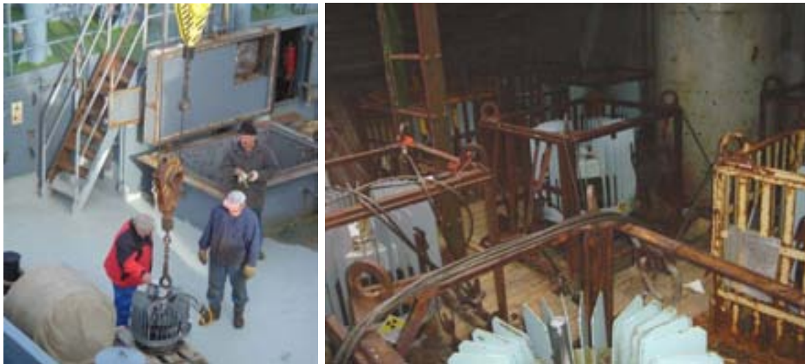
Fig. 7. The RTG packages are unloaded from the pontoon by the ship's crane. RTG packages are placed and fixed in the ship's hold or on deck in locations that are the most distant from the ship's crew temporary or permanent attendance of the personnel.
