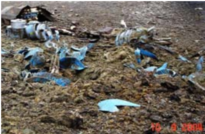
Fig. 13. Photo of the two dropped RTGs of the type Efir-MA, Tiksi hydorraphic base.
