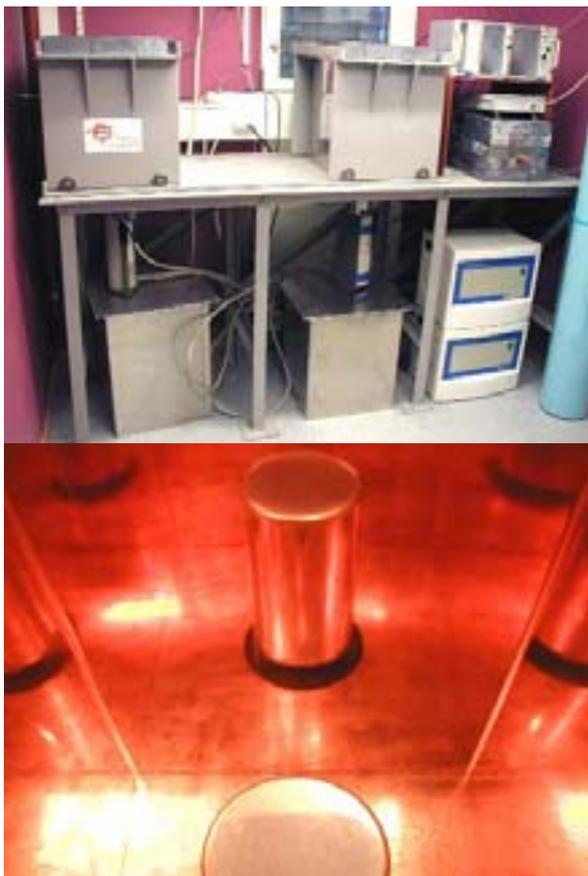
**Figure 1.1** Two electrically cooled HPGe detectors and shielding at the laboratories of the NRPA, Tromsø (top), close up of an HPGe detector inside a copper/tin lined lead shield (bottom).
