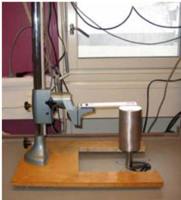
**Figure 3.5.** Measurement of point sources for detector characterisation.
