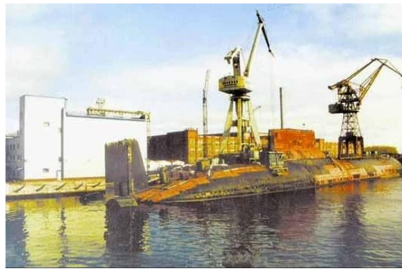
Fig. 2.1.3. "Typhoon" class NPS being dismantled at "Sevmash" berth.
