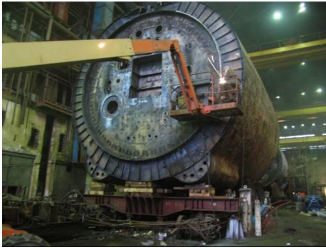
Fig. 2.6.3. Preparation of the reactor compartment from dismantled Project 705 nuclear sub with titanium hull at "Nerpa" shipyard.
