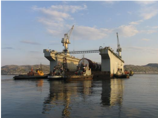
Fig. 2.6.5. Reactor compartment shipment from "Nerpa" shipyard to Saida LSF on board "Pallada" floating dock.
