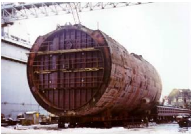
Fig.2.6.1. Three-compartment reactor section from dismantled NPS in a floating dock
