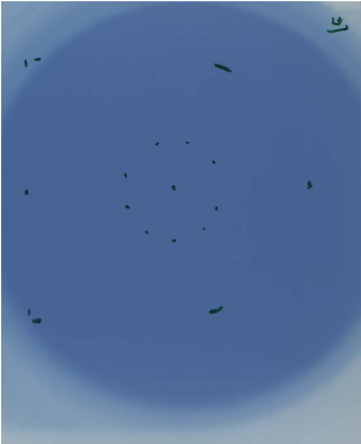
Figure 3: Raw Gafchromic EBT image showing the field relative to the marks present on the irradiation shelf in the cabinet.
